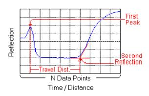
**Figure 1:** Basic principles used by WinTDR for analysis of a waveform.
